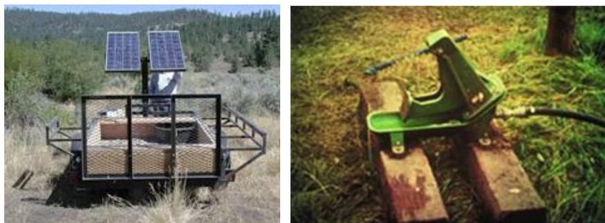
Figure 10. Creating upland water sources with a mobile solar powered pump (left) and nose pump mounted on railroad ties (right).
